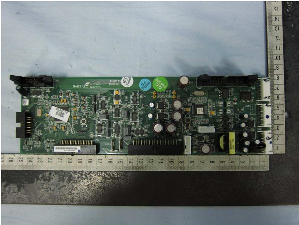
Control Board_Solder side view
