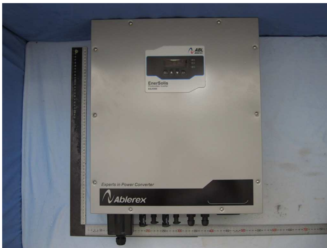
Inverter (ES 5500T, Alternate construction) AC-DC section
