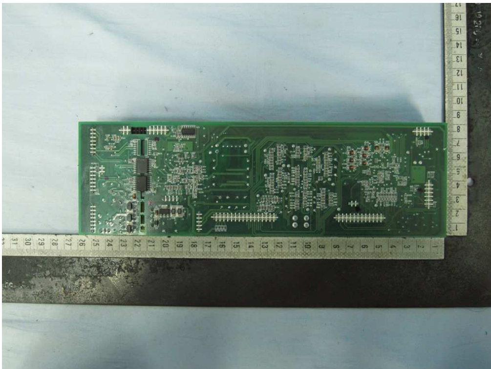
Control Board_Solder side view
