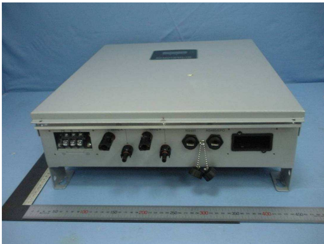
Inverter (ES 5000H) AC-DC section
