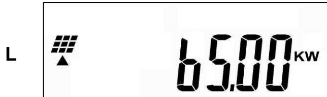
6.2.6 Output power of booster B
